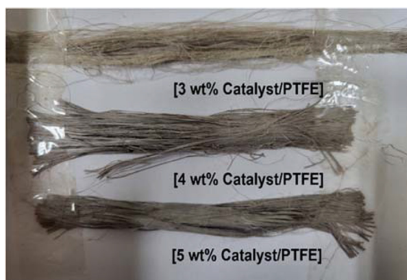
Fig. 3. PTFE fibers prepared with different amounts of NO removal catalyst.
